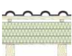
31 cm Polystyrol (30 kg/m 3 )
